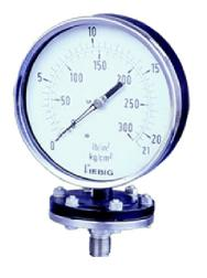
These guages are suitable for use on corrosive gases and liquids. Diaphragm Materials of Stainless steel with Teflon protection; Case Material of pressure die cast aluminium, steel or stainless steel. Wetted parts of Stainless Steel, Mild Steel. Available in all standard process connections NPT, BSP etc; Accuracy  $\pm$  1% Dial Size 100mm and 150mm. Pressure Range from 40 millibar to 600 millibar and 0-1 kg/cm<sup>2</sup> upto 0-21 kg/cm<sup>2</sup>. Also Vacuum and Compound.
