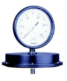
These gauges are suitable for low pressure measurement of non-corrosive gases, commercial heating, gas distribution and filtration. Measuring System of Brass or SS 304 Capsule. Case Material cast aluminium. Available in pressure range 0-50 mm WC upto 1000 mm WC in pressure, vacuum and compound ranges. Available in all standard process connections NPT, BSP etc.; in dial sizes 100 mm and 150 mm Accuracy  $\pm$  2%.
