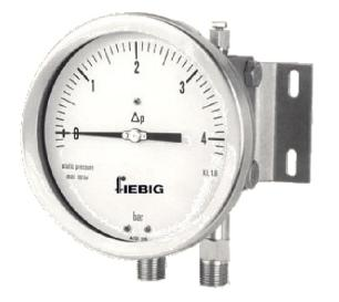
Consisting of two bourdon tubes, one for high and one for low pressure line and the pointer of the instrument gives direct reading of differential pressure. Each bourdon tube can take maximum pressure of 1.3 times the maximum range shown on the dial. Manufactured in dial size 150mm and with pressure range from 0 - 1 kg/cm<sup>2</sup> upto 1000 kg/cm<sup>2</sup> and with accuracy  $\pm$ 1%.
